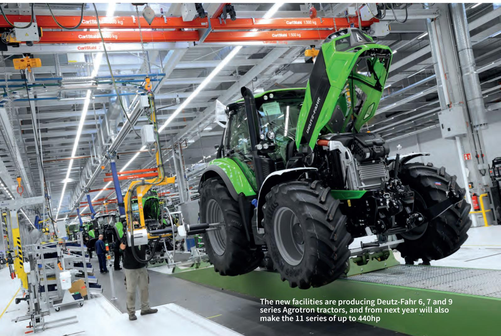
The new facilities are producing Deutz-Fahr 6, 7 and 9 series Agrotion tractors, and from next year will also make the 11 series of up to 440hp
