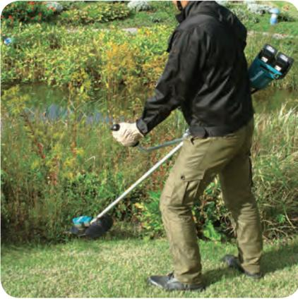
The new Makita DUR365UZ 36v cordless brush cutter features the company's brushless motor in the cutting head which it says is a major advancement in performance, reduced weight and improved balance.
