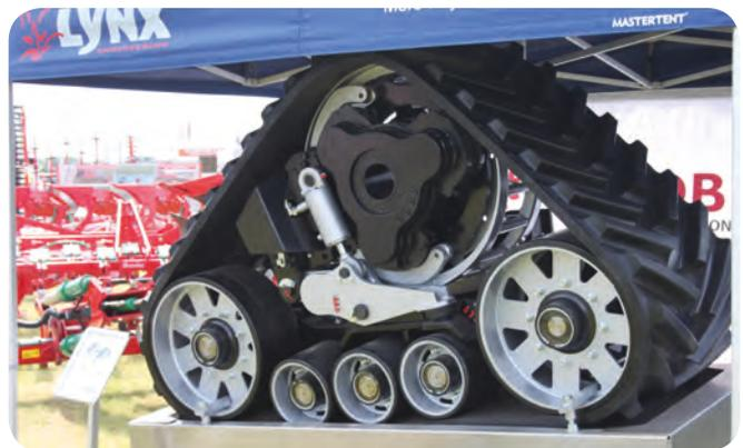
Retro-fit rear track units have found homes with a number of UK cropping businesses seeking increased traction and flotation from high-hp tractors yet wanting a fully wheeled tractor at other times of the year, but the downside for many is the 40% reduction in road speed that they impose. Lynx Engineering is now offering a new 40km/hr (25mph) rated system from Dutch maker Zuidberg.
