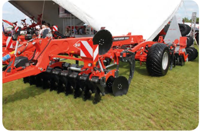
Cultivation and drilling equipment from bigger names included a 3m version of Kuhn's Performer deep-working disc/tine cultivator. Key components include two rows of 510mm independent and hydraulically adjustable discs and four rows of non-stop hydraulic breakback tines capable of working to a maximum depth of 350mm. Tine point choices include standard 80mm shares, 50mm subsoiling shares or wing shares. At the rear is a notched roller providing up to 225kg/m of hydraulically adjustable pressure.
