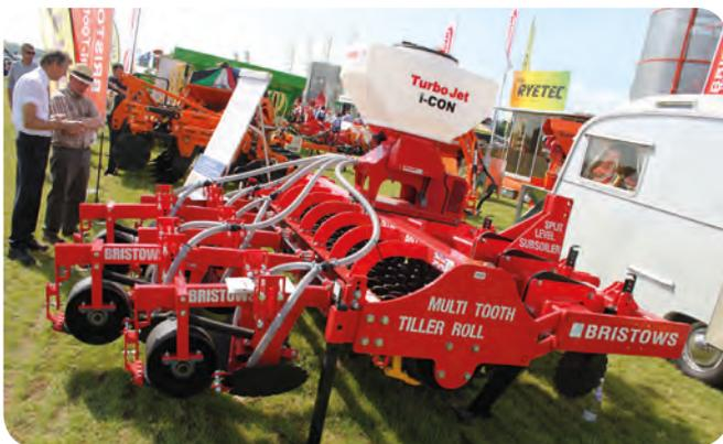
Simplicity was also a theme with the Split-Level subsoiler from Bristows, a firm based not far from the Cereals site. Targeted at the oilseed rape establishment market, it can be specified with leading loosening tines or discs, which precede subsoiler legs of various types depending on the level of shattering and surface movement required.
