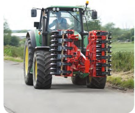
tractor when attached, ensuring that it follows the nose of the tractor, steering smoothly even at speed. The headstocks are designed to take the forces produced even when using a shattaboard.
