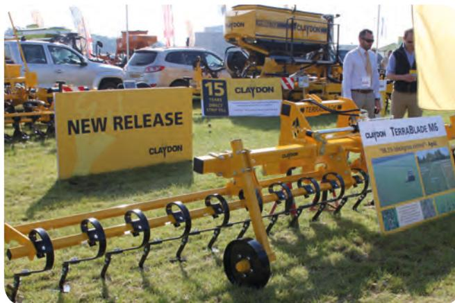
Making its debut on the Claydon stand was the firm's front linkage-mounted Terrablade inter-row hoe, designed for shallow working between wide-row band-sown crops established using one of the company's drills to reduce demands on herbicides and cut crop protection bills. Claydon says the Terrablade can be used at forward speeds of approximately 6.0km/hr, working at up to 20mm deep. Guide wheels are installed at the front of the implement.
