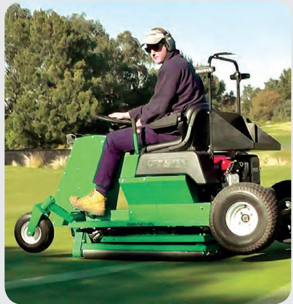
Charterhouse Turf Machinery launched a new turf roller from Graden.
