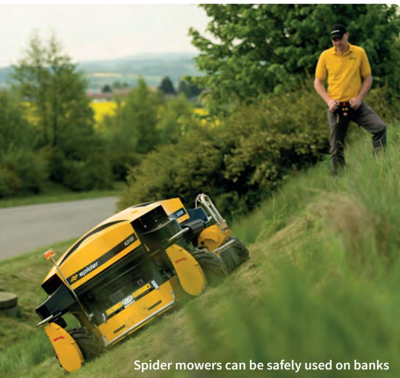
Spider mowers can be safely used on banks
