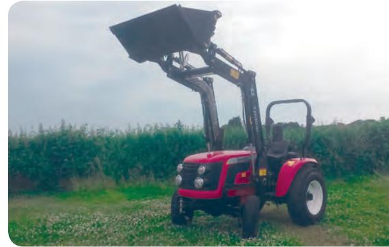
which is a self-levelling loader designed specifically for the 254CH.
