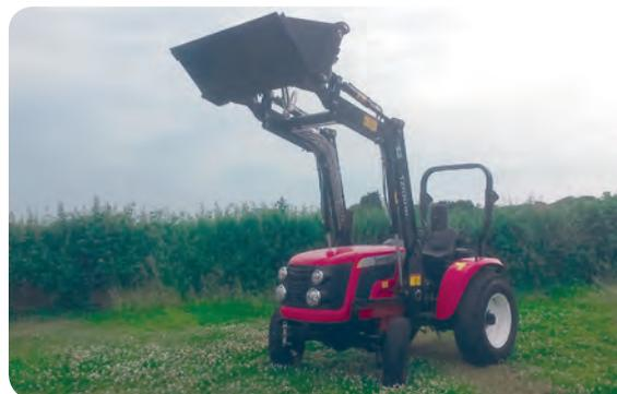
which is a self-levelling loader designed specifically for the 254CH. The loader offers a lift capacity of 400kg and a digging depth of 140mm. The bucket has a 0.2 m<sup>3</sup> capacity.
