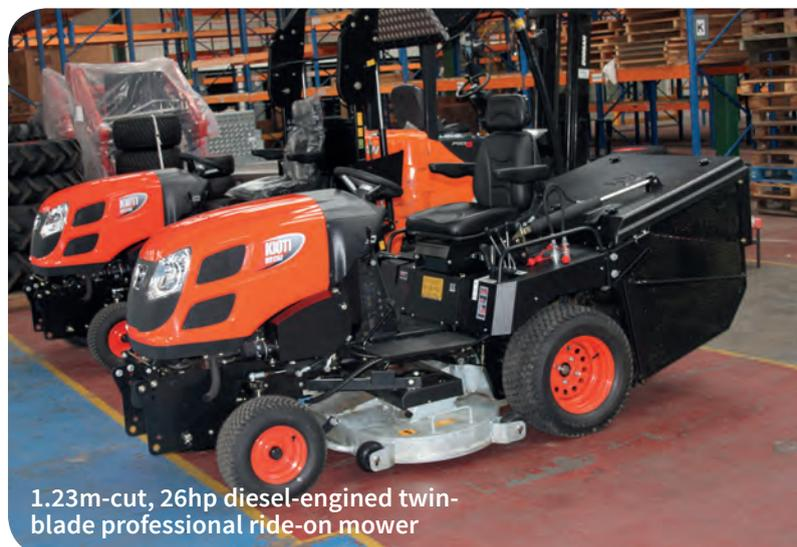
1.23m-cut, 26hp diesel-engined twin-blade professional ride-on mower
