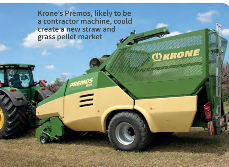
claims output is up to 5.0t/hr, three to five times the output of most traditional 'fixed' pelleting systems.
