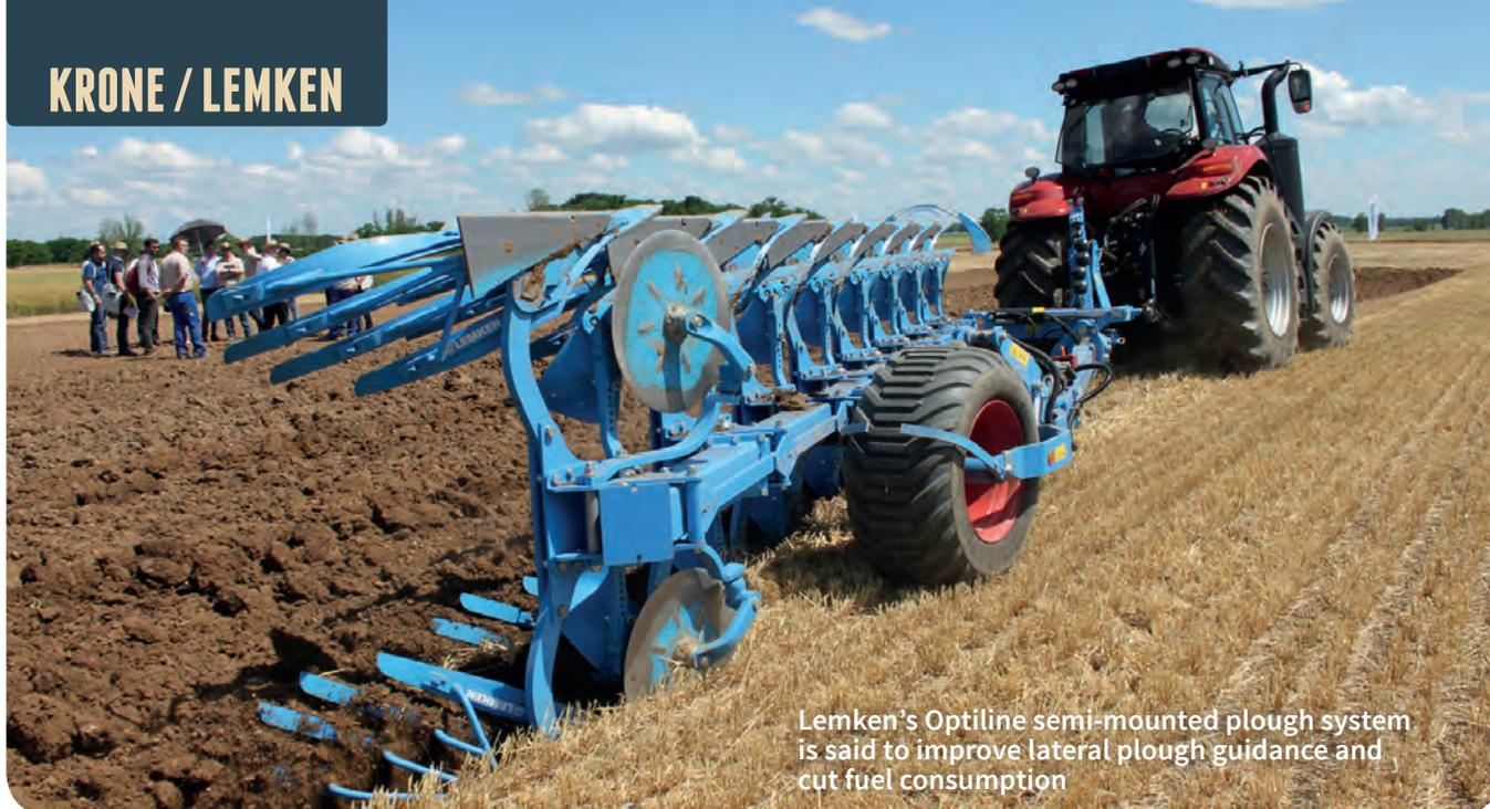
Lemken's Optiline semi-mounted plough system is said to improve lateral plough guidance and cut fuel consumption
