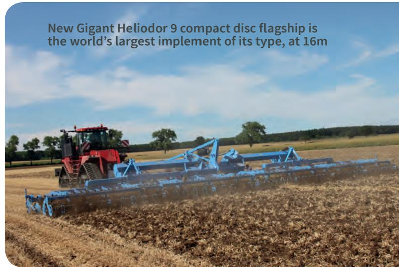
New Gigant Heliodor 9 compact disc flagship is the world's largest implement of its type, at 16m
