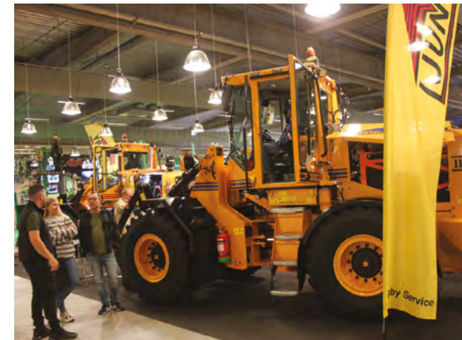
Electric drivetrain version of L11 wheel loader from Ljungby
