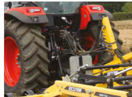
Standard rear spec comprises a 4.4t rear linkage, two double-acting mechanical spools and 540/540E/1,000rpm PTO
