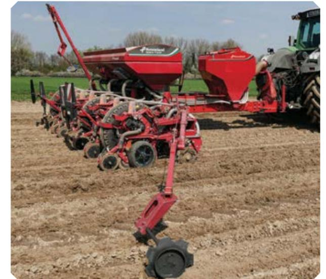
"One seed injector per row is located at the bottom of the seed hopper, and air is used from the fan to transport seed to the sowing units at the back of the drill," he says. "Seeds carried in the airstream collect in a buffer area directly above each sowing heart, where a 1.5-litre seed tank holds a ready-supply of seed for each unit."
