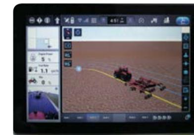
**AFS Connect allows A-B lines and other data to be planned on a farm PC and transferred wirelessly to the tractor. Owner and dealer monitoring is also possible**
