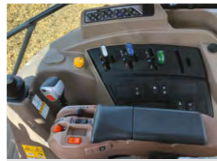
Cab spec is kept simple, with mechanical spool valves, but there is an armrest with integrated hitch and throttle controls
