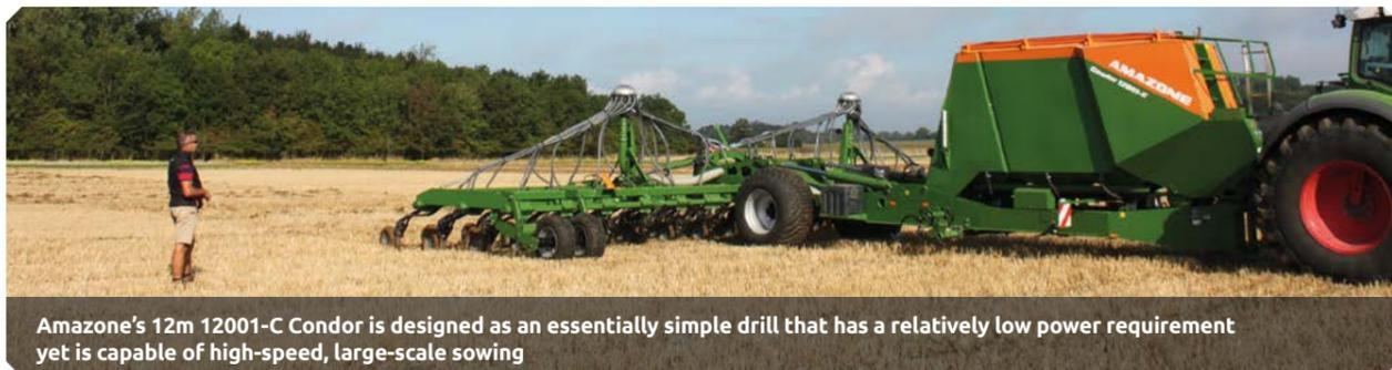
Amazone's 12m 12001-C Condor is designed as an essentially simple drill that has a relatively low power requirement yet is capable of high-speed, large-scale sowing
