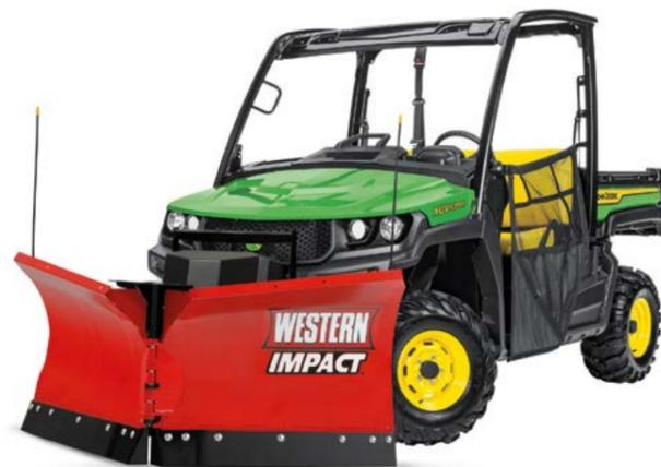
There is a choice of 1.82m (72in) straight and V-blade snow plough models with hydraulic or winch lift, and each comes with replaceable cutting edges and plough markers. The hydraulic blades feature an in-cab joystick control for lifting and angling, and optional accessories include plough shoes, rubber deflectors or poly cutting edges.
